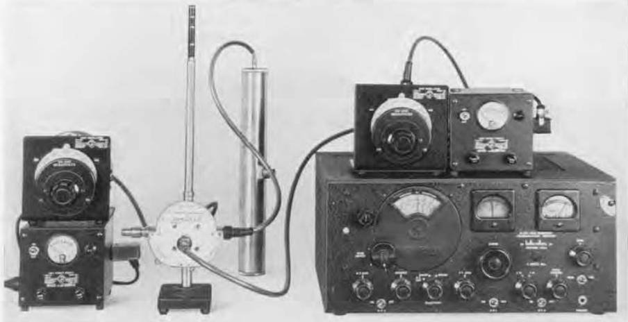
Figure 5. View of the admittance meter in use with standards and unknown connected. The generator is a Type 1208-A Unit Oscillator and the null detector is a communications-type receiver, with a second unit oscillator and Type 874-WM Mixer acting as a frequency converter. The unknown admittance being measured is an u-h-f transformer.
