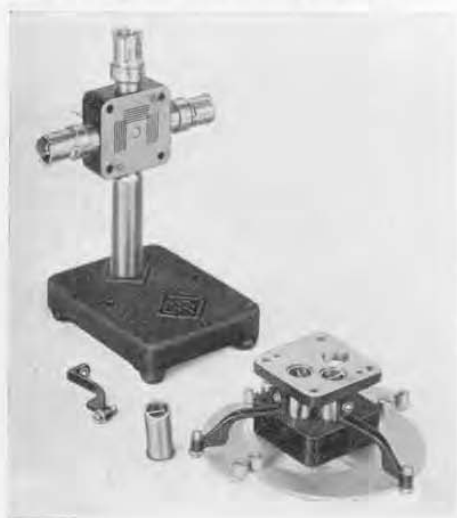
Figure 4. View showing internal parts of the admittance meter. The pickup-loop assembly has been removed from the generator junction assembly to show the coupling slots and the coupling loops.
